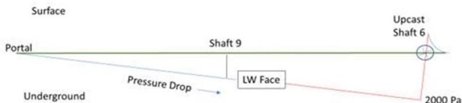
If it is assumed that shaft 9 is located around halfway in the ventilation circuit (pressure drop wise) and if shaft 9 is capped, around -1000 Pa may be measured across the shaft collar.
