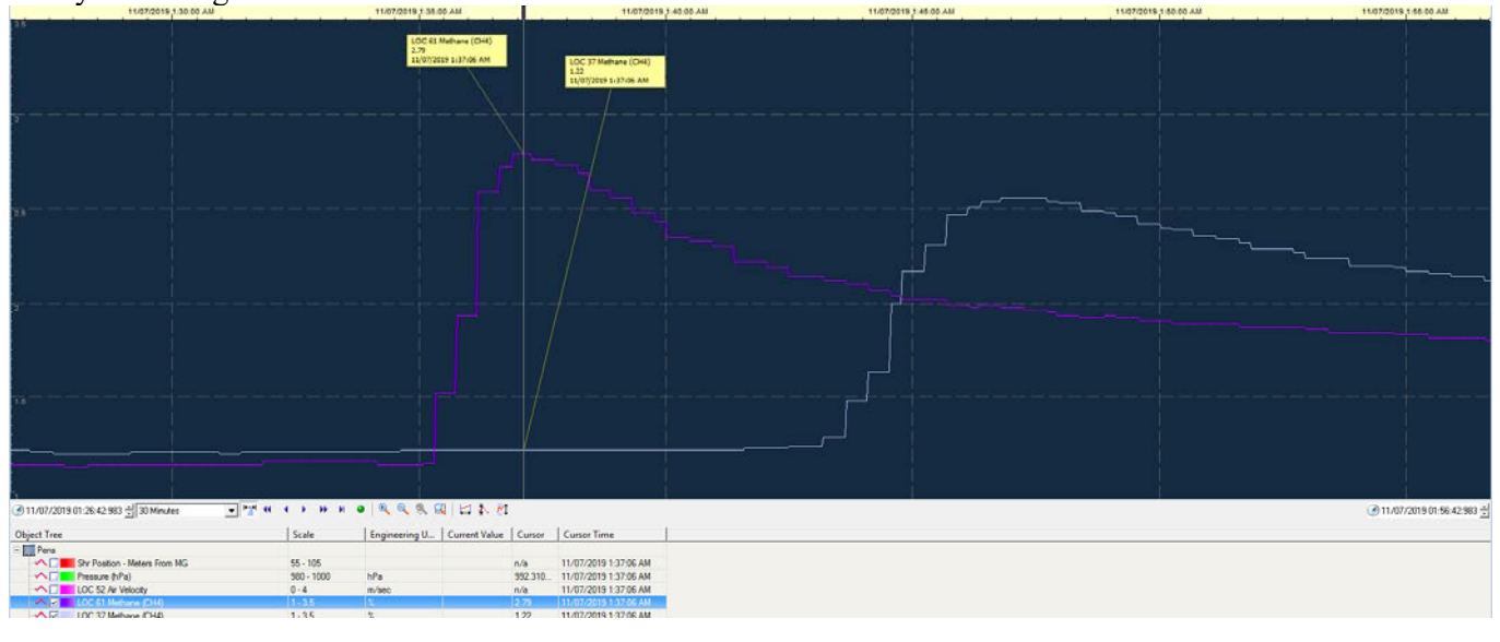
Graph showing time that the CH4 sensors in the TG were reading greater than 2.5% CH4 Inbye Sensor greater than 2.5% for 3min Outbye Sensor greater than 2.5% for 2min
