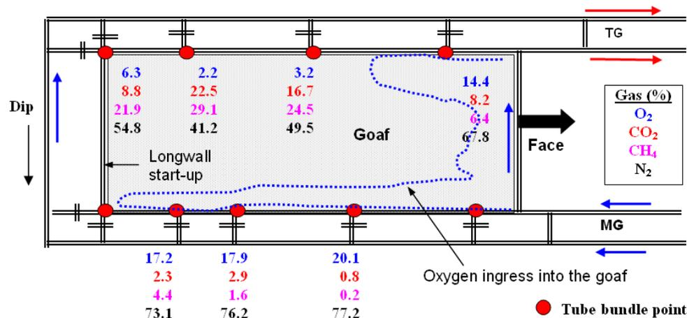
Fig.1. Typical gas distribution in a longwall goaf
