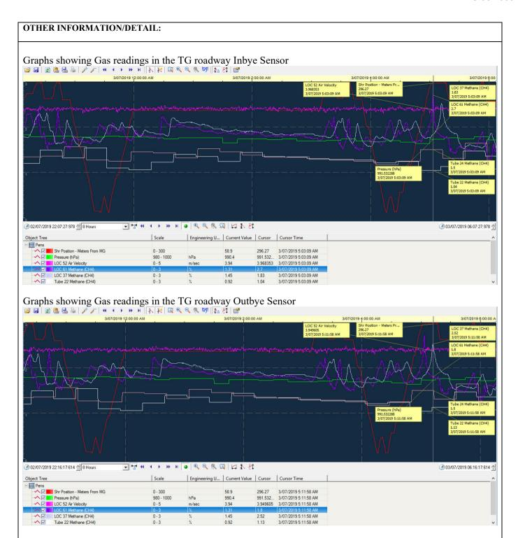
After the event, production was stopped to allow the gas levels to reduce to an acceptable level before the TG was advanced and shearer moved to a safe location. Plan for the next 36hrs is to develop a plan to improve TG CH4 management prior to production recommencing.
